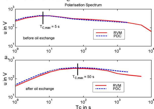
**Fig. 8** Polarisation spectra determined by PDC analysis and recovery voltage measurement (RVM) from measurements
