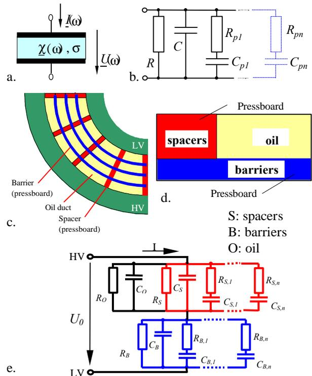
**Fig. 2** a. Plate capacitor as a model for dielectric arrangements
