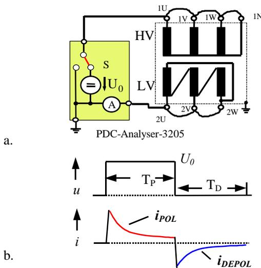
**Fig. 1** a. Measurement of the relaxation currents using the Siemens measuring system PDC-Analyser-3205 [3]
