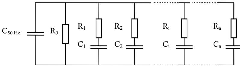
**Figure 1:** Equivalent circuit to model a linear dielectric
