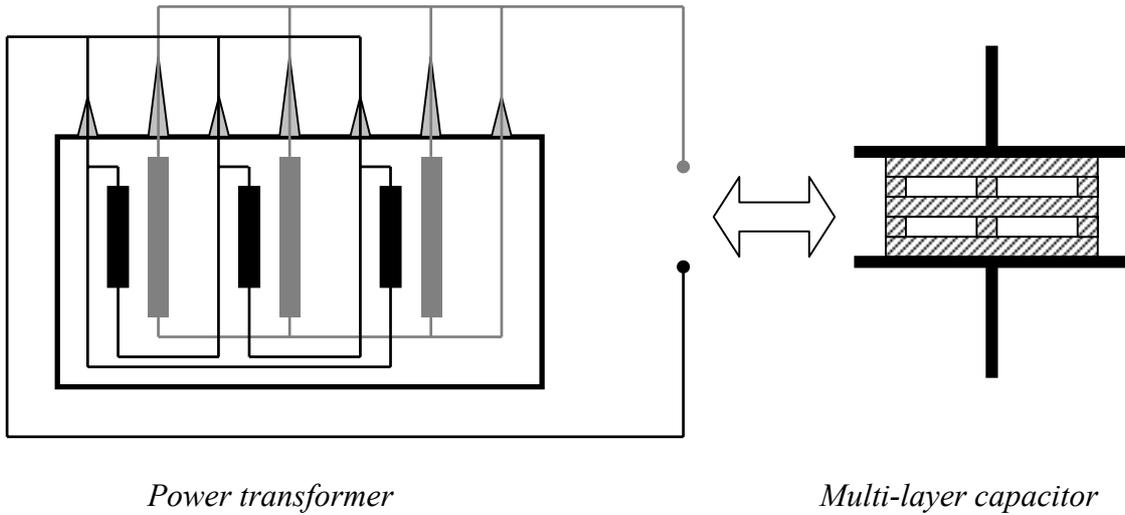
Figure 2: How to connect a power transformer as capacitor for the dielectric investigation of the main insulation.
