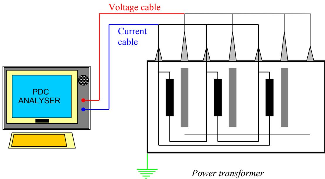
Figure 3: Connection of a power transformer to **PDC-ANALYSER-1MOD**.
