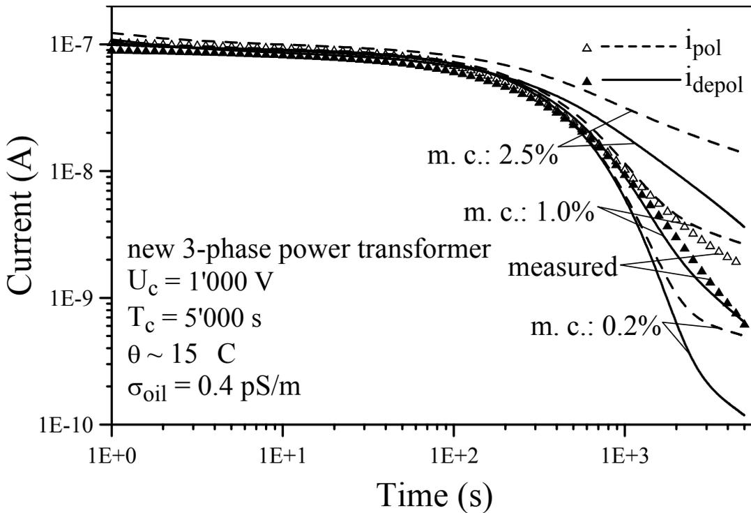
Figure 2: Comparison between measured and calculated relaxation currents as a function of moisture content (m. c.) in the pressboard barriers and spacers of a power transformer.
