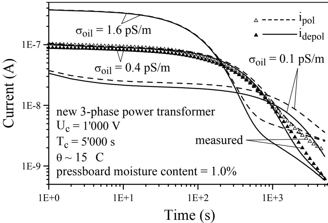
Figure 1: Measured and calculated relaxation currents as a function of oil conductivity  $\sigma_{oil}$  of a new power transformer.
