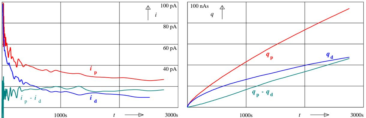
**Fig 1:** PDC measurement on OIP bushing no. (3) from fig. 7 (left): Currents and current differences, CDM charge difference method (right): Total charge  $q_p$ , stored charge  $q_d$  and non-stored charge  $q_p - q_d$ .
