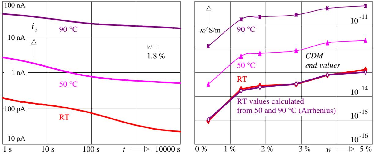
**Fig.3:** Polarisation currents at different temperatures through OIP samples with 1.8 % water (left) and d.c. conductivities calculated from charge differences (CDM values) as function of temperature and water content (right). RT values are additionally calculated from 50 and 90 °C for verification of Arrhenius' law (right, empty symbols).  $E = 0.1$  kV/mm, oil no. 1.
