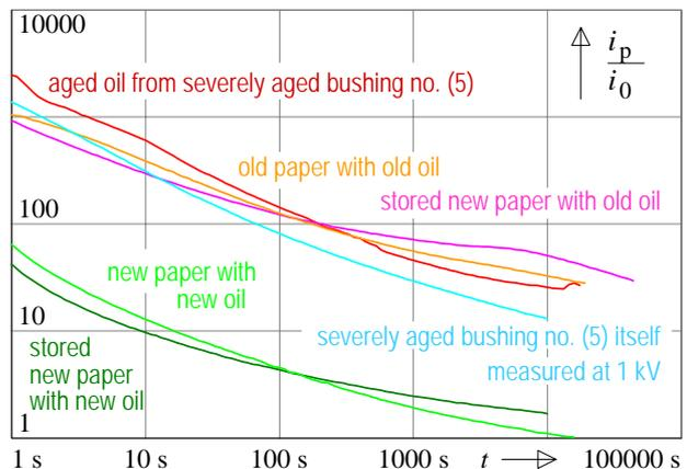
**Fig. 8:** Influence of service aged oil on polarisation currents in OIP. Currents are normalized to the same capacitance, measured at RT and 1 kV/mm.
