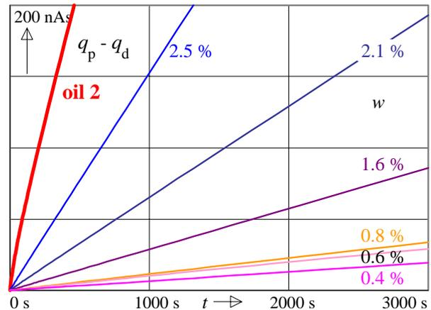
Generally it is possible to distinguish different water contents with PDC measurements directly, fig. 4. Best differentiation is given for long measuring times. For short times  $< 300$  s no differences were observed between 1.3 and 2.8 %.
