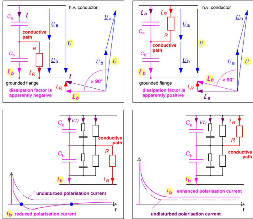
right). A conductive path to ground can result in a temporary discharging of  $C_b$ , in a negative current  $i_b$  and in two polarity reversals, fig. 10 (left).
