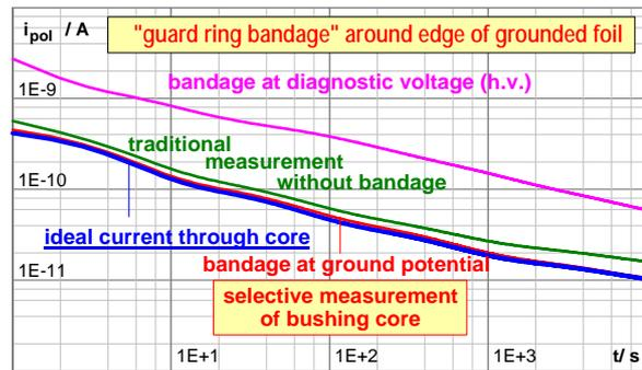
derived from PDC measurements on material samples for all materials used in a bushing. The results of simulations are in good agreement with measurements, fig. 12 (top right and left). Only small current differences could be observed, probably because material samples and bushing materials are not absolutely identical. The bushing was a spare object and stored for 10 years.
