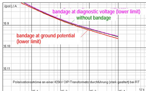
**Fig. 13:** Polarisation currents measured on a severely aged 420 kV OIP bushing no. (5) in fig. 7 and table 1, measured at RT and 1 kV.
