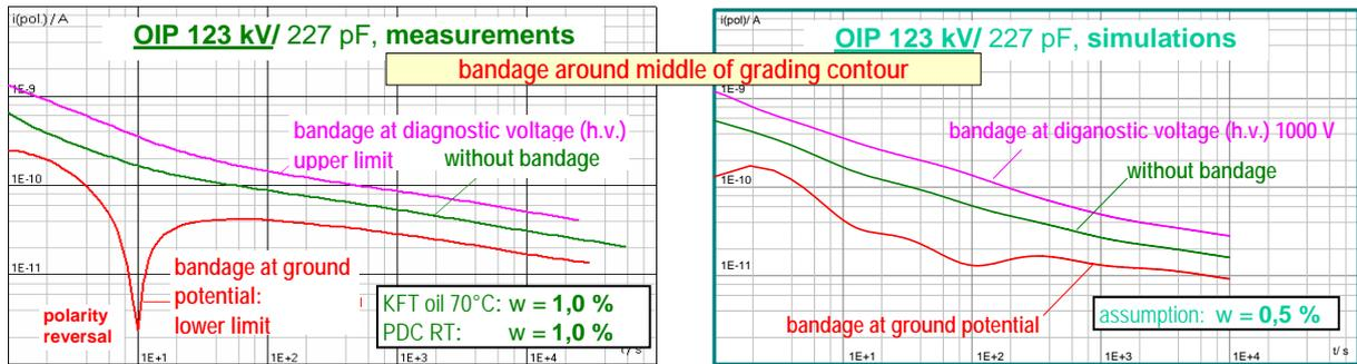
**Fig. 12:** PDC measurements without and with bandages in the middle of the grading contour. Bandages at h.v. and ground give upper and lower limits for polarisation currents through the bushing's core (**worst case bandages**), measurements (*top left*) and simulations (*top right*).
